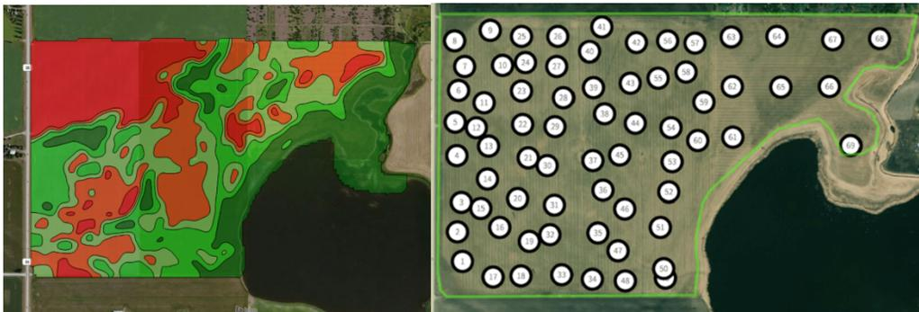
*Figure 2 - Map of soil zones (n=37) used to predict pH in the Hubbard field trial 2018-2021 (left) density of data points (n=69) collected using hyperspectral approach resulting in heat map for precision lime application (right)*
