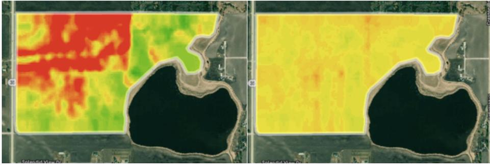
*Figure 3 - pH heatmap created using hyperspectral approach (Left) vs heatmap previously used using zoned sampling approach (Right).*
